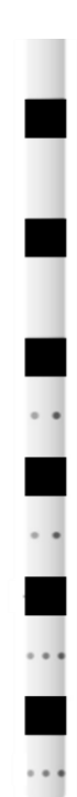
Figure 1. The schematic of temporary SEEG electrode implanted in target regions. Black squares represent macro/stimulation contacts while little circles represent micro contacts.
